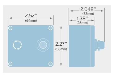
REMOTE PCA ENCLOSURE FOR HIGH TEMPERATURE TRANSMITTERS (2 meter interconnect cable, not shown)
