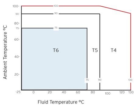
**Note:** Consult factory to determine the functional temperature limit of your transmitter variant. Temperature class ratings do not correspond with the continuous duty area for the electronics within the transmitter. A complete description of your transmitter may be found on the Max Machinery web site (www.maxmachinery.com). Individual specification sheets and product family manuals are also available for viewing or downloading.
