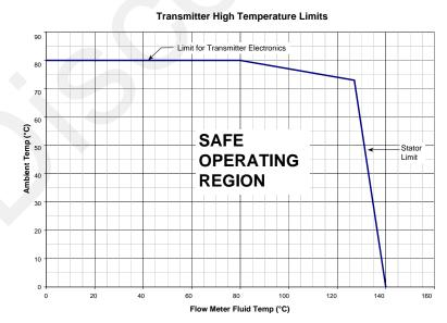
The stator of the 286 transmitters is insulated with an electrical coating that is rated to 130°C which limits the maximum flow meter fluid temperature to about 130°C (265°F).
