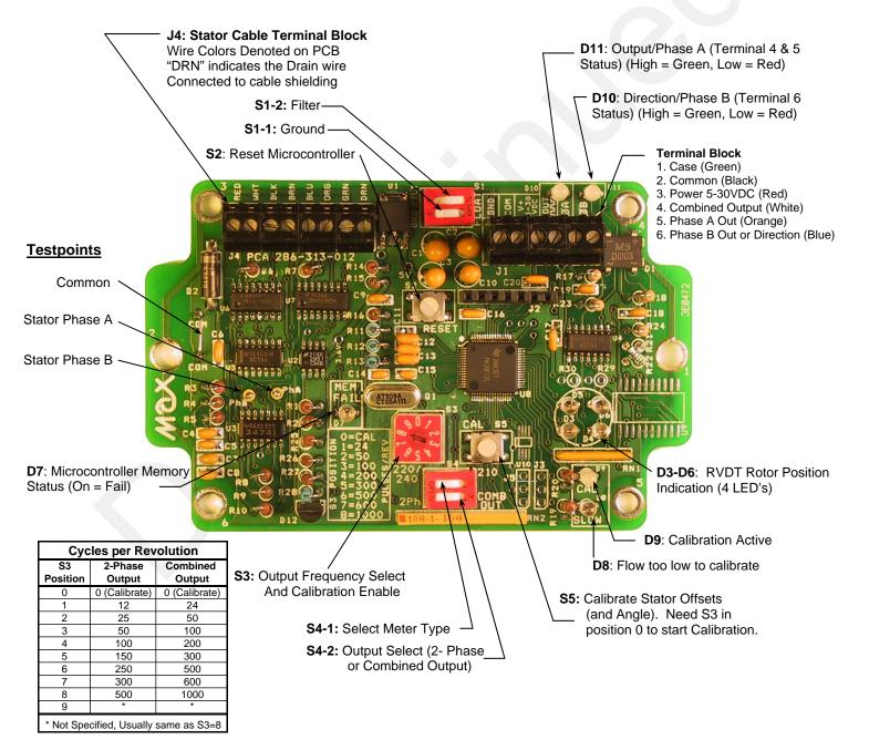
286-314: Transmitter with Amphenol Connector, Level Shifter Option
